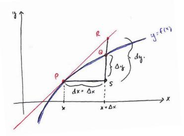
Notice the corresponding change in **y** is  $\Delta y = f(x + \Delta x) - f(x)$  *dy* represents the amount that the tangent line rises or falls, whereas  $\Delta y$  represents the amount that the **curve**, y = f(x) rises or falls when **x** changes by an amount *dx*. *dx* always =  $\Delta x$  but *dy* is just an approximation of  $\Delta y$ .
